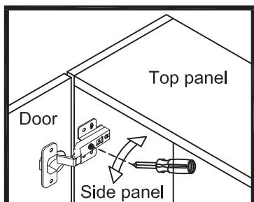
Loosen or tighten the screw indicated a little to adjust the gap between doors panels (see step 3a & step 3b)
