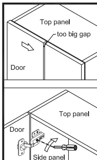
Turn the screw clockwise a little as shown to make the gap small.
