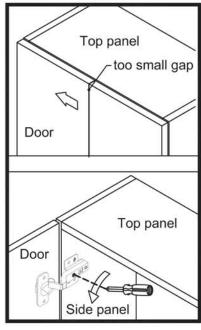
Turn the screw counterclockwise a little as shown to make the gap big.
