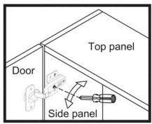
Loosen or tighten the screw indicated a little to adjust the gap between doors panels (see step 3a & step 3b)
