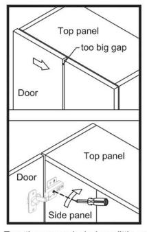
Turn the screw clockwise a little as shown to make the gap small.
