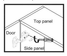
Loosen the screw indicated a little, adjust the hinge to right position (see step 2a & 2b), then tighten the screw.
