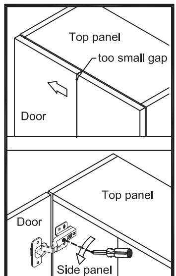
Turn the screw counterclockwise a little as shown to make the gap big.
